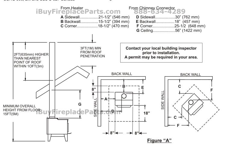
Unit must be placed on a noncombustible floor protection equivalent to 3/8" millboard extending 18" (457mm) in front and 8" (203mm) to side and back of unit per manufacturer's instructions. Consult your local building authorities for further information.
